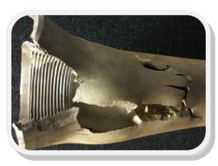
The above images are examples of the empirical testing undertaken to validate our severing tool performance at 450 °F. Note how the physical test is also validated by that of the FEA shown in the above strain plot images.
