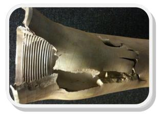
The above images are examples of the empirical testing undertaken to validate our severing tool performance at 450  $^{\circ}$ F. Note how the physical test is also validated by that of the FEA shown in the above strain plot images.
