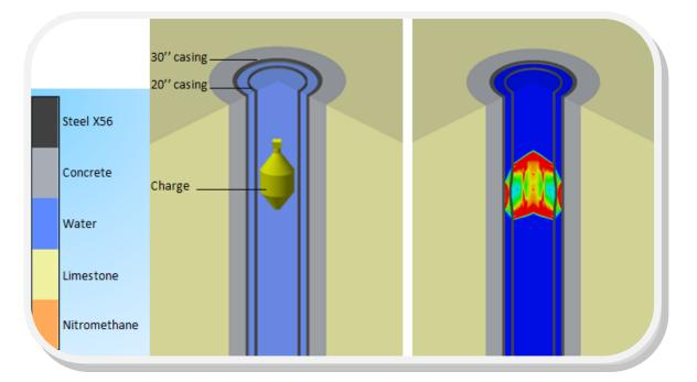
SPEX has the capability to simulate explosive events, to predict severance capability and optimise the explosive charge weight required.
