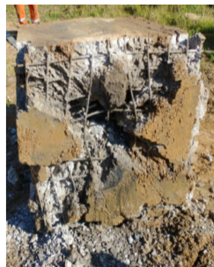
1m 3 Concrete Test Block - Post Detonation
